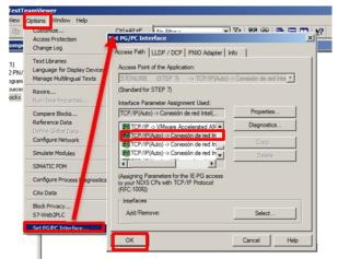
To set the type of communication in the Simatic software, one has to open the dialog in "Options" and select "Set PG/PC interface" and select the type of communication between the PLC and the PC, which normally appears as the name of your Ethernet card installed in the Computer. There is usually an option for every existing adapter on the computer (usually Ethernet and wireless card).
