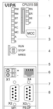
The vast majority of the S7 PLC incorporate an Ethernet interface for communication with the connected equipment. This interface is generally located in the CPU module (item 6). An
